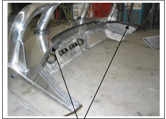
Figure 12 – Attach 6mm black clip lock trim to centre and infills to either side
